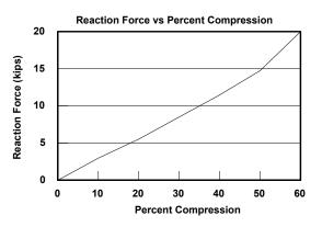
\*Above information is for our Standard Capacity *Marine Guard*<sup>™</sup> foam filled marine fenders. Actual values for all sizes may vary plus or minus 15% from stated values due to variations in material properties, dimensional tolerances, temperature and speed of compression.
